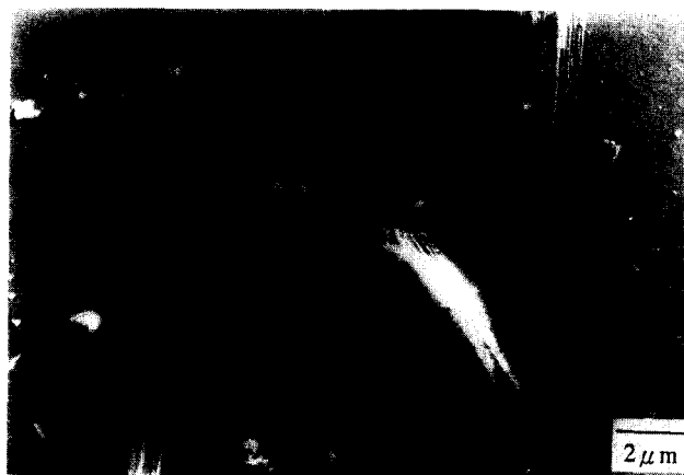
Figure 1 PLLA crystals precipitated by isothermal crystallization of the 0.08% (w/w) solution in acetonitrile at 25°C
